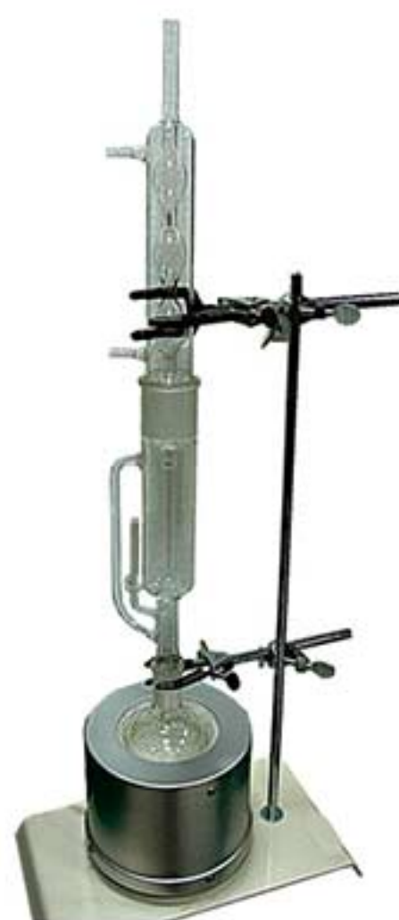
2. 含油轴承含油量Soxhlet (沙格利特)萃取设备
